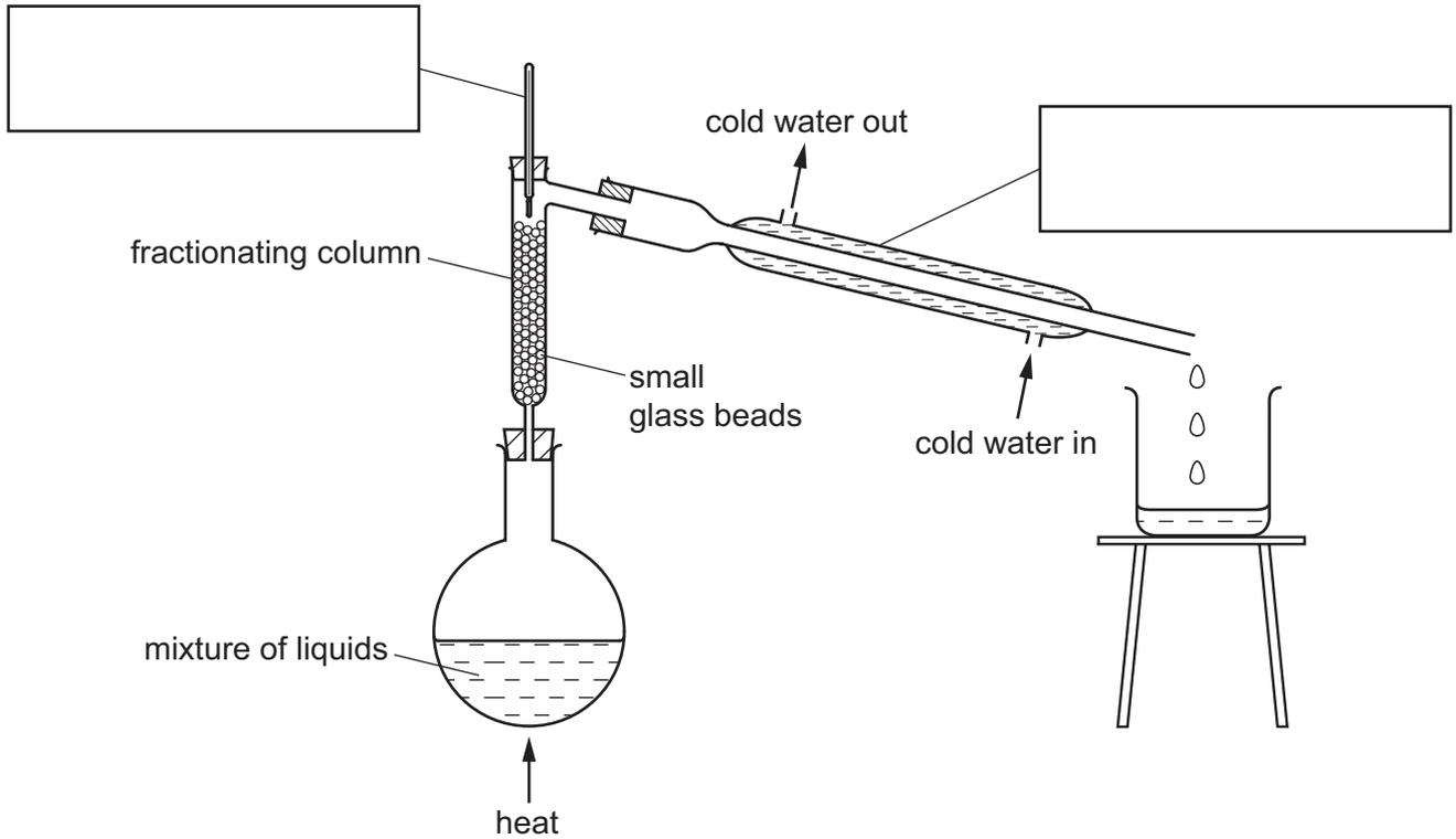
(a) Complete the boxes to label the pieces of apparatus used. [2]
